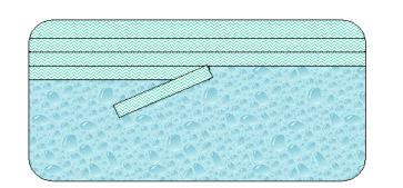
Cut patch a minimum of 100mm larger than 3 the damaged area. For larger patches allow at least 200mm extra. Radius corners. Remove strips of backing paper to reveal adhesive.
