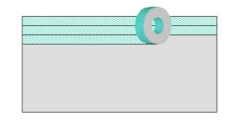
Lay out patch film on flat surface. Affix 2 transfer tape to patch (side by side) until entire patch is covered. Ensure all air bubbles are rolled out.
